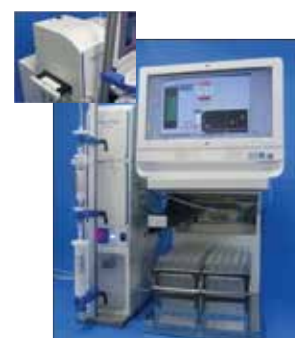
SmartFlash AKROS Built-in TLC Image Reader chromatography
